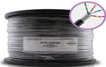
**CABLE UTP CAT5E ENSON 13151B305 DOBLE FORRO SERIE PRO-II CALIBE 24 AWG 100 COBRE BOBINA DE 305 METROS FORRO PE COLOR NEGRO Y PVC COLOR GRIS USO EXTERIOR RECOMENDADO PARA CCTV VIDEO IP Y REDES BASE 10100**
