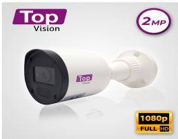
**CAMARA HD BULLET TOPVISION TBFC200A AHD / TVI / CVI /SD / 2MP / 2.8MM / 30M LUZ CÁLIDA / MICROFONO INTEGRADO / IP67 / COC / CARCASA PLÁSTICA / 12VDC IMAGEN A COLOR 24X7 AUDIO POR COAXIAL O UTP**
